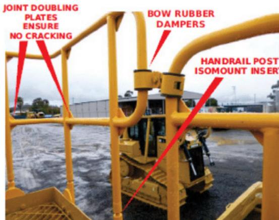
"HANDRAIL POST ISOMOUNTS" & BOW RUBBER DAMPERS ELIMINATE VIBRATION .
